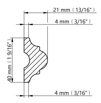
kovex www.kovex.co.uk @ sales@kovex.co.uk **L** +44 (0) 1823 77 44 00 Product type: Railing Product name: Classic Railing 32 Product code: Kovex CR32 Product measurements: Length: 2440 mm Width: 40 mm Projection: 21 mm Scale: 1:1 Do not scale All dimensions in mm (inches) All information contained in this document is
